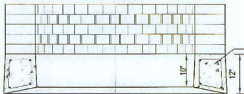
ALTERNATIVE RING FOUNDATION TO PROTECT SINK PIT IN LOOSE SOIL
